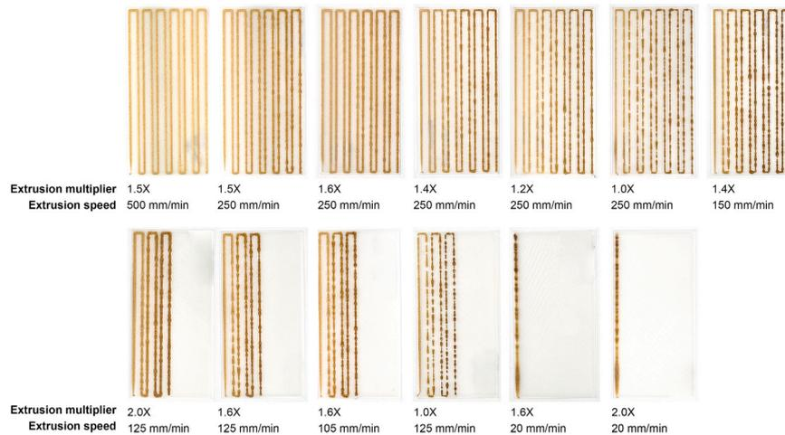
Fig. A.3. Gradient exploration by extruding wood filament for 1500 mm with variable printing speed and extrusion rate. The nozzle temperature is initially set to 195°C and heats up to 300°C while extruding the material.
