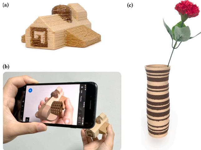
**Fig. 11.** a) Body portion of a toy car with an AR marker printed on the front. b) AR overlay of the front nose and of a textured wheel using Adobe Aero app. c) A flower vase with a 1D barcode incorporated as a functional esthetic element.
