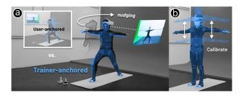
Figure 5: Implementation of *Trainer-anchored* layout: (a) the *Trainer-anchored* layout is nudging a user to alter posture while the *User-anchored* layout is following the user. (b) A virtual trainer is calibrated to the user's height.
