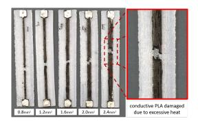
Figure 3: All five samples were damaged by excessive heat
