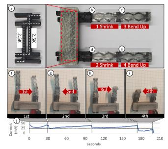
Figure 17: (a) Parallel connection with conductive material (b-e). Planned sequential activation of four cells, step-by-step actuation (f-i), and a graph showing when fuses blow (j)
