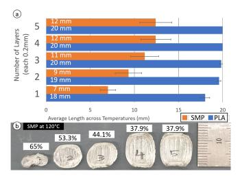
Figure 1: (a) Average length of SMP and PLA samples with different number of layers after being heated, and (b) average shrink rate with representative five heated geometries
