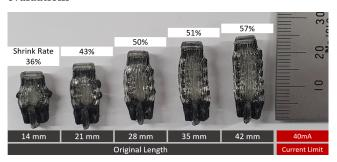
Figure 11: Maximum shrink rates for varying length and 40 mA max current threshold
