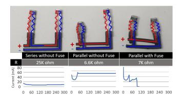
Figure 13: Naïve coupling of *ShrinkCells in-series* and *in-parallel* result in incorrect actuation vs. preventing overheating with a fuse mechanism (right)
