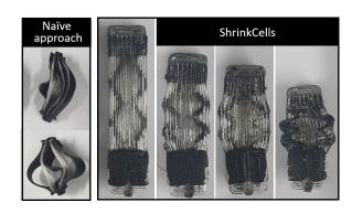
Figure 6: Buckling behavior of SMP layers when naïvely heated vs. ShrinkCells's folding behavior
