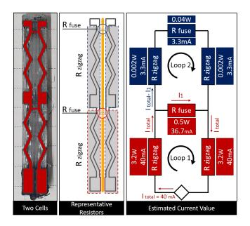
Figure 16: Schematic diagram on two connected cells showing the current flow in two cells placed in parallel. The current values are estimated by measuring the resistance of the zigzag structure and fuses of the *ShrinkCells* after printing (R-zigzag = 2000  $\Omega$ , R-fuse = 400  $\Omega$ ).
