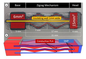
Figure 7: (a) Construction details of a *ShrinkCell*, and (b) layering PLA and SMP material
