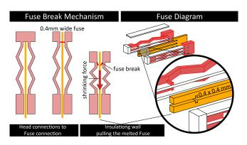
Figure 14: The fuse mechanism  $(0.4\times0.4 \text{ mm})$  connects two zigzag structures instead of the head  $(15 \text{ mm}^2)$ . The shrinking force of an insulating wall pulls down and breaks the fuse, stopping the current flow and the cell's shrinkage.
