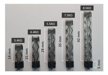
Figure 10: Five samples of *ShrinkCells* used in the technical evaluations
