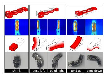
Figure 8: Five different actuation by selective heating of the zigzag mechanism
