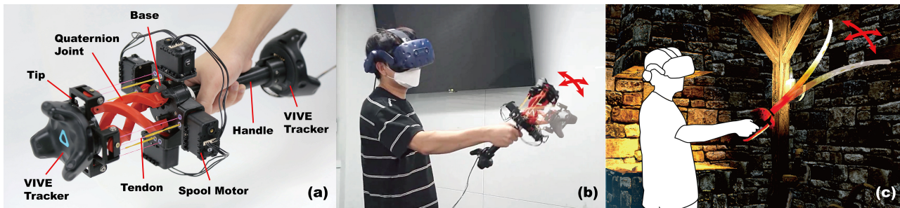
Figure 1: (a) ElaStick prototype and components, (b) user interaction with the ElaStick physical controllers, which is mapped to a flexible sword in virtual reality (c).
