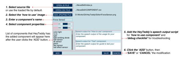
Fig. 5. The graphical software used to create and customize the behavior of additional components.
