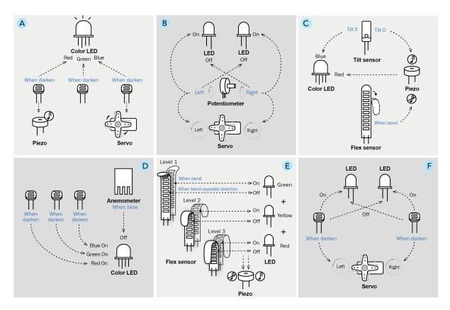
Fig. 7. Diagrams for the six prototypes used in the modality study. Users were given similar tasks consisting of controlling actuators (motors, LEDs, piezo) given some input from sensors (photoresistor, flex sensor, anemometer).
