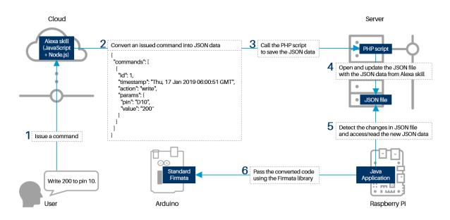
Fig. 6. Overview of the software process from the issued command to the execution of instructions on the Arduino.
