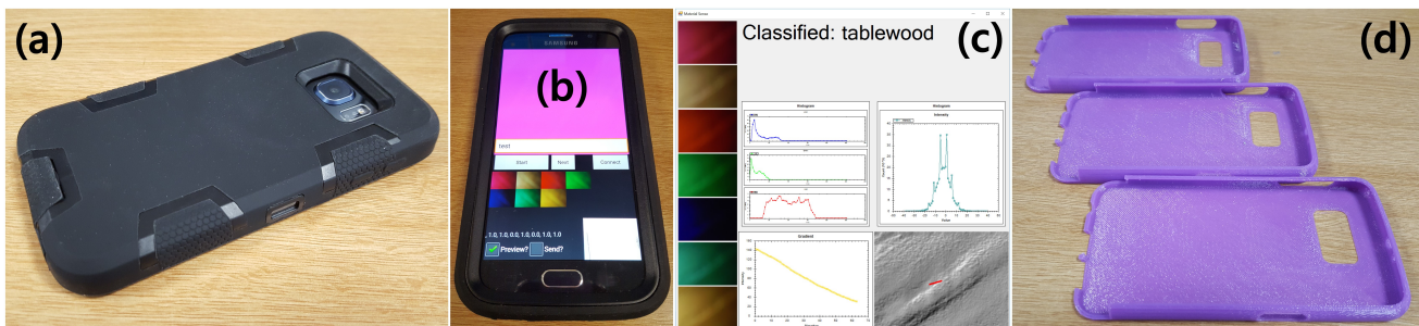
Figure 1. a) The phone is facing down while the screen flashes different colors and the camera captures images of the reflected light. b) The UI of the phone, showing the main light source and the captured images. c) The UI of the classification server, showing the received images, the classification results on top and the extracted features (color histogram, gradient, etc). d) 3D printed cases with different height for the pilot study.
