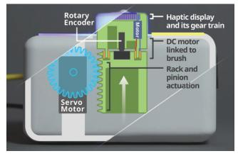
Figure 3. Rack and pinion actuation, brushing, and gearing required for the haptic display.
