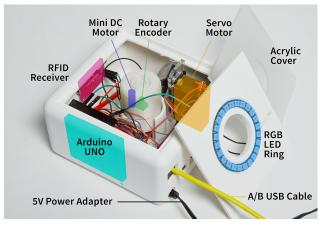
Figure 2. Button+ internal components and assembly.
