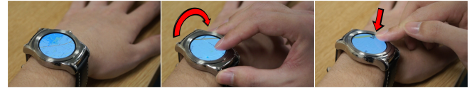
Figure 5. Map application running on LG watch Urbane: Twist to zoom and pressure touch to move the map at different speed.
