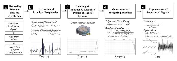
Figure 2. RealPen algorithm for generating the tactile sensations of pen-writing.
