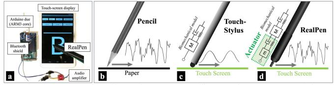
Figure 1. RealPen recreates the writing-sensations corresponding to different types of pens based on the analysis of friction-induced oscillations and sound of real pen tips moving on paper.
