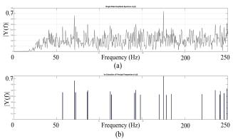
Figure 4. a) FFT result, b) extracted principal frequencies.
