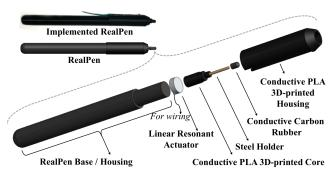
Figure 3. Implemented RealPen and its schematic illustration.
