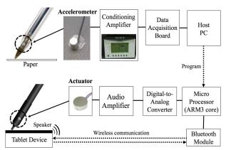
Figure 6. Hardware of RealPen setup.
