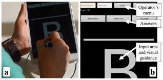
Figure 9. (a) Experimental set up used to test the auditorytactile perception and (b) the GUI for the first part of the study.
